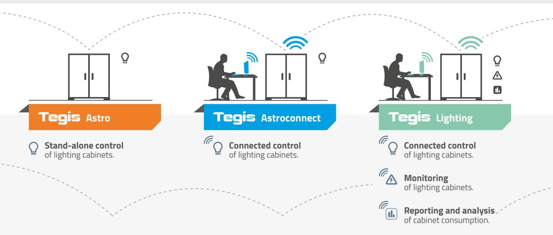
Cabinet control (energy and maintenance savings): the control is the primary source of energy savings thanks to its integrated astronomical clock. The connected astronomical clock makes remote configuration possible.
